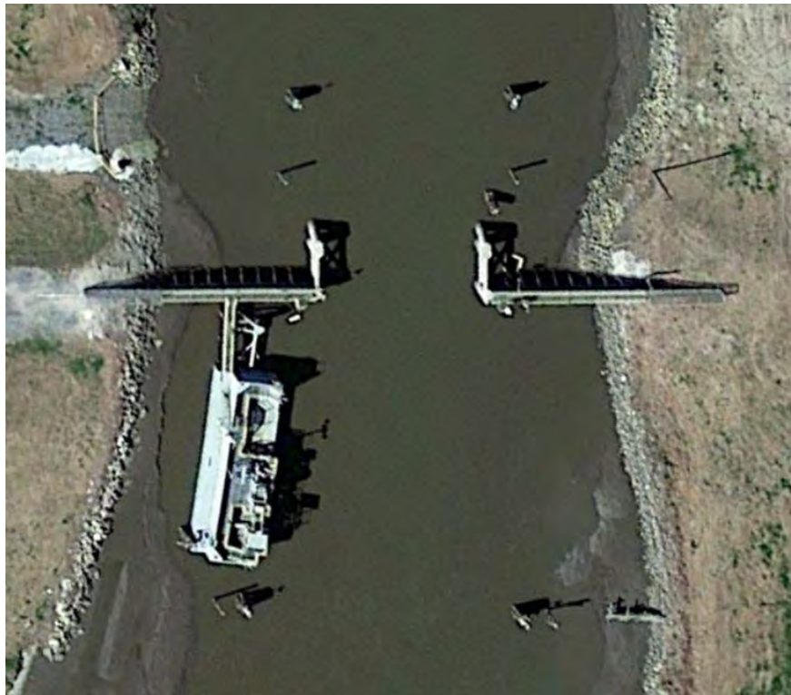
Figure 2: Typical Barge Gate Example
