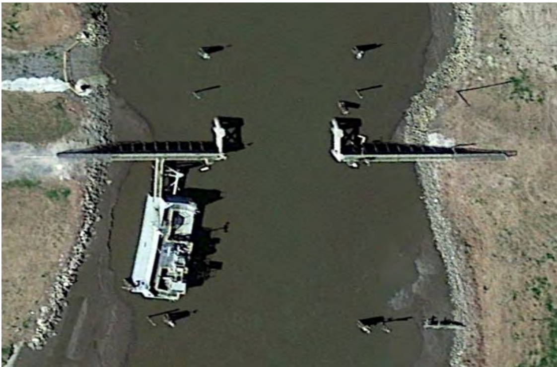
Figure 2: Typical Barge Gate Example
