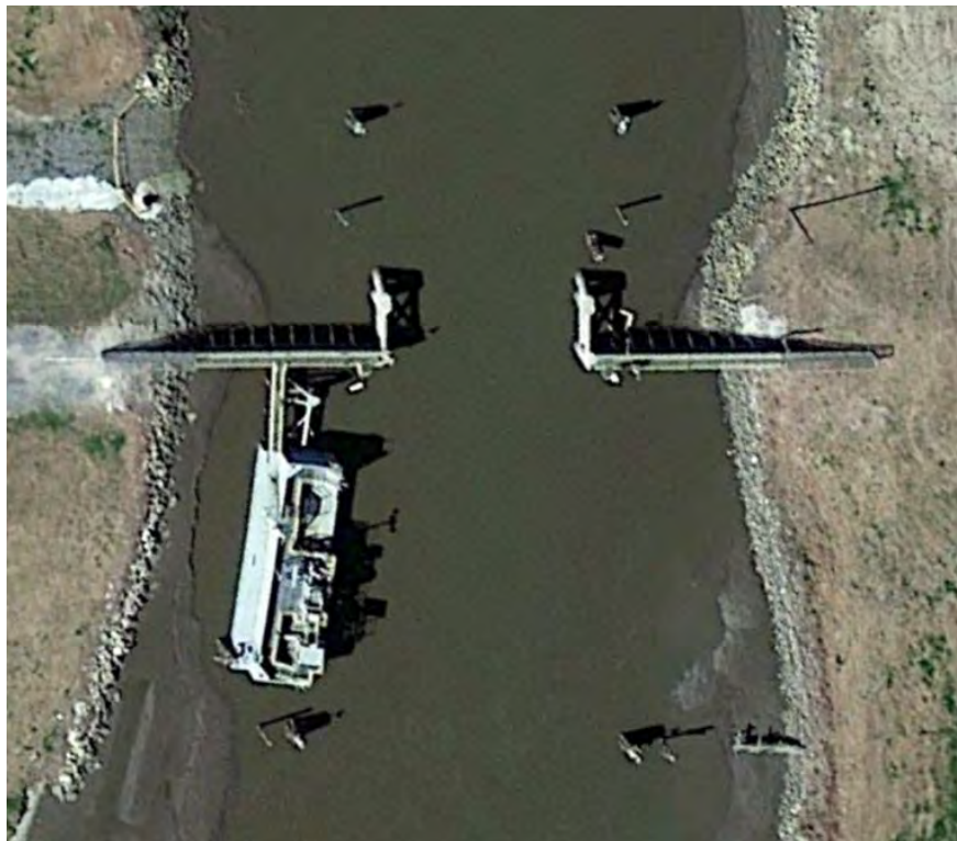
Figure 2: Typical Barge Gate Example
