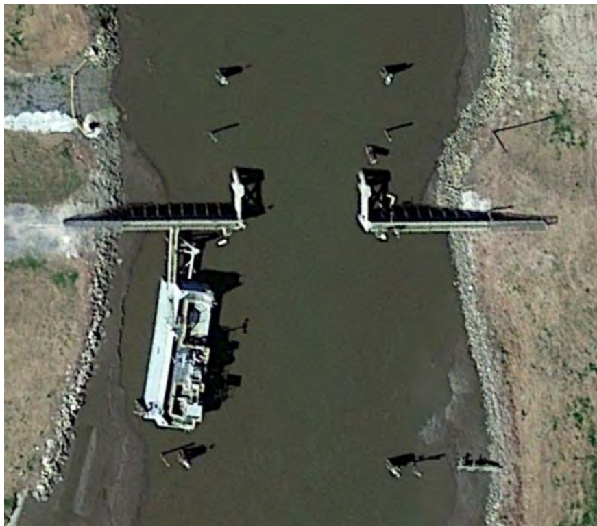
Figure 2: Typical Barge Gate Example
