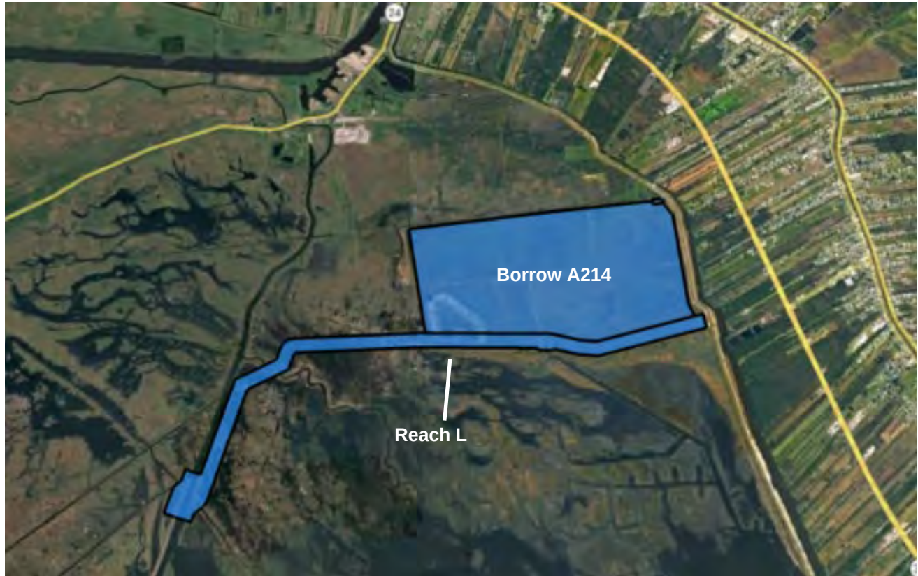
Figure 4. Reach L borrow site and haul route.
