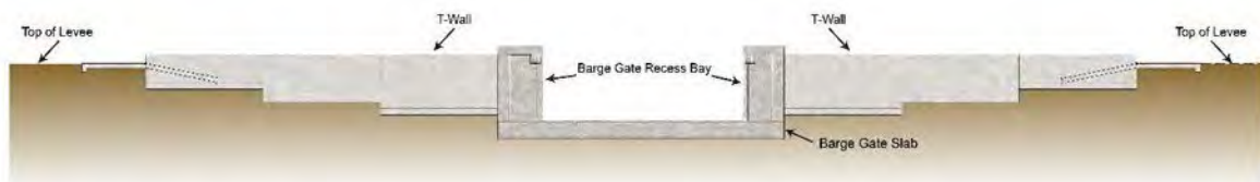
Figure 3: Conceptual Barge Gate - Elevation View with Gate in Open Position
