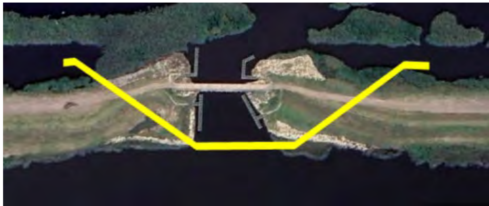
Figure 5. Potential floodside alignment of floodwall segment
