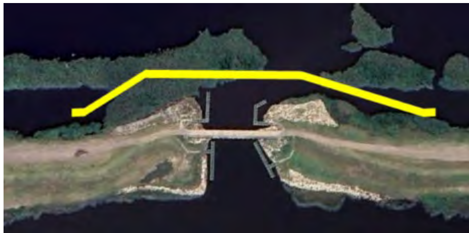
Figure 6. Potential protected side alignment of floodwall segment
