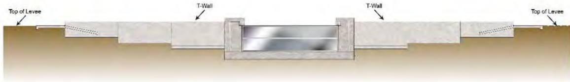
Figure 3: Conceptual Stoplog Gate - Elevation View with Gate in Open Position (Crane not shown for clarity)
