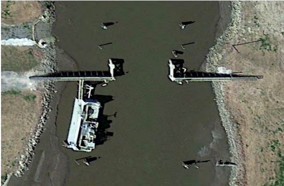
Figure 2 – Typical Barge Gate Example
