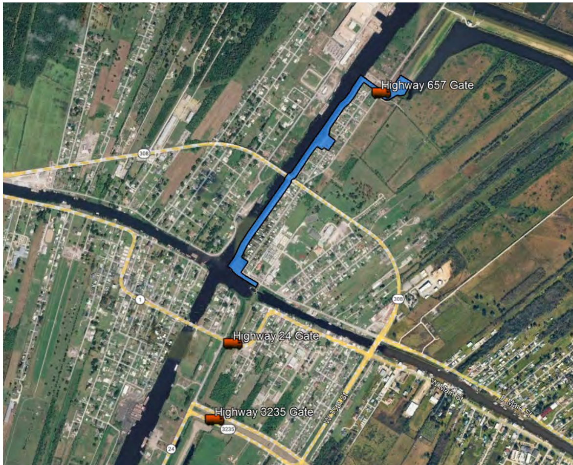
Figure 2: GIWW Floodwall (blue) and Highway Gates (red)
