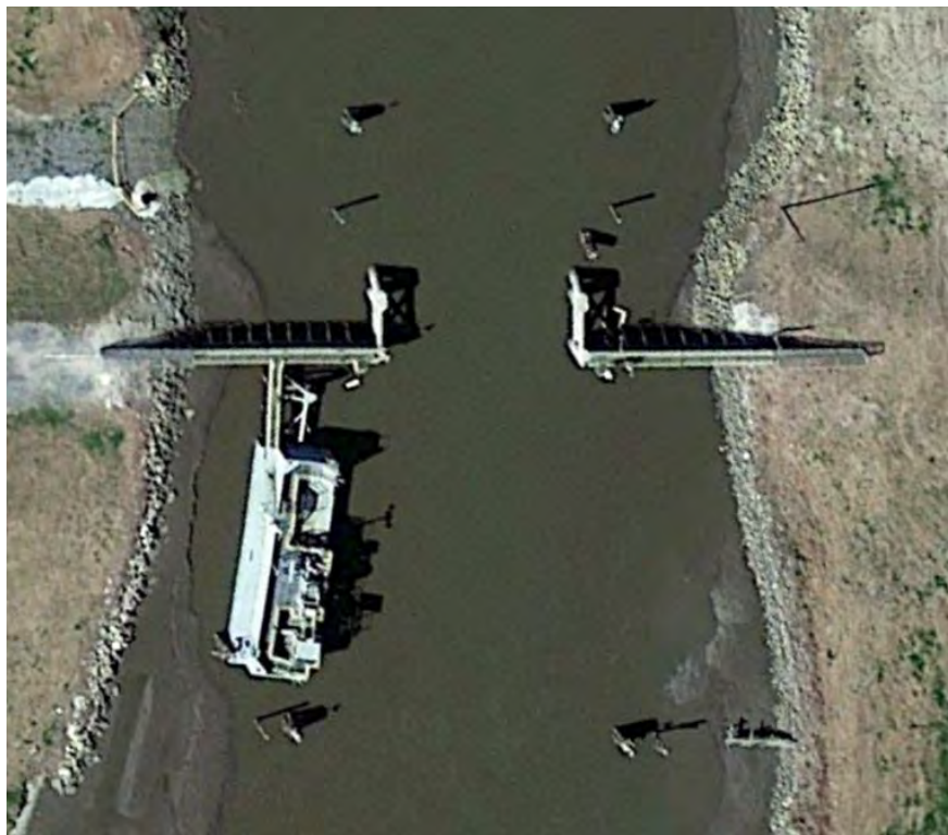
Figure 2: Typical Barge Gate Example
