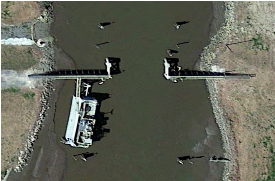
Figure 2: Typical Barge Gate Example
