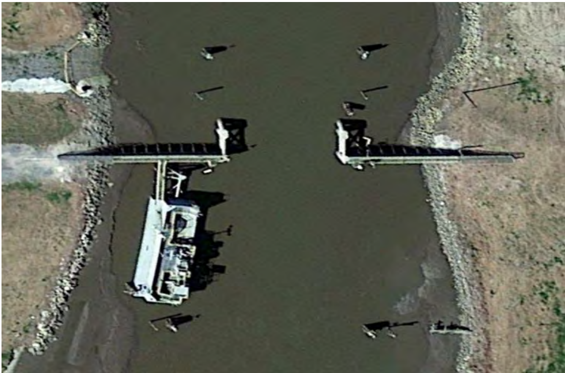
Figure 2 – Typical Barge Gate Example
