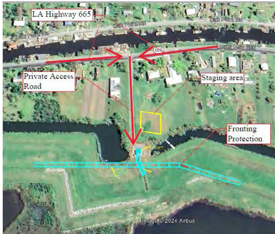
Figure 5: Access and Staging
